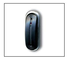
MIFARE® DESFire® ISO14443A (13,56 MHz) card proximity reader with read/write capability. This reader allows the CSN (Chip Serial Number) of the card to be read, as well as read/write operations of data in the card memory.
