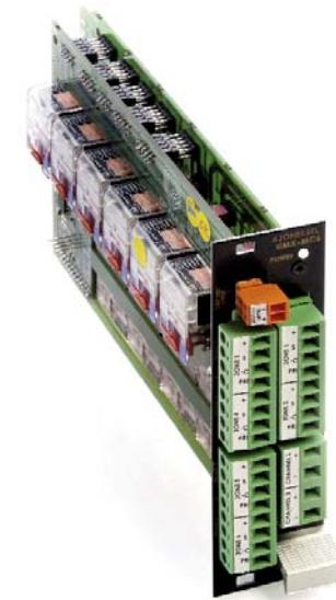
The UMX-MC6 card can be inserted into the free slots of the COMPACT and COMPACT-E units.
