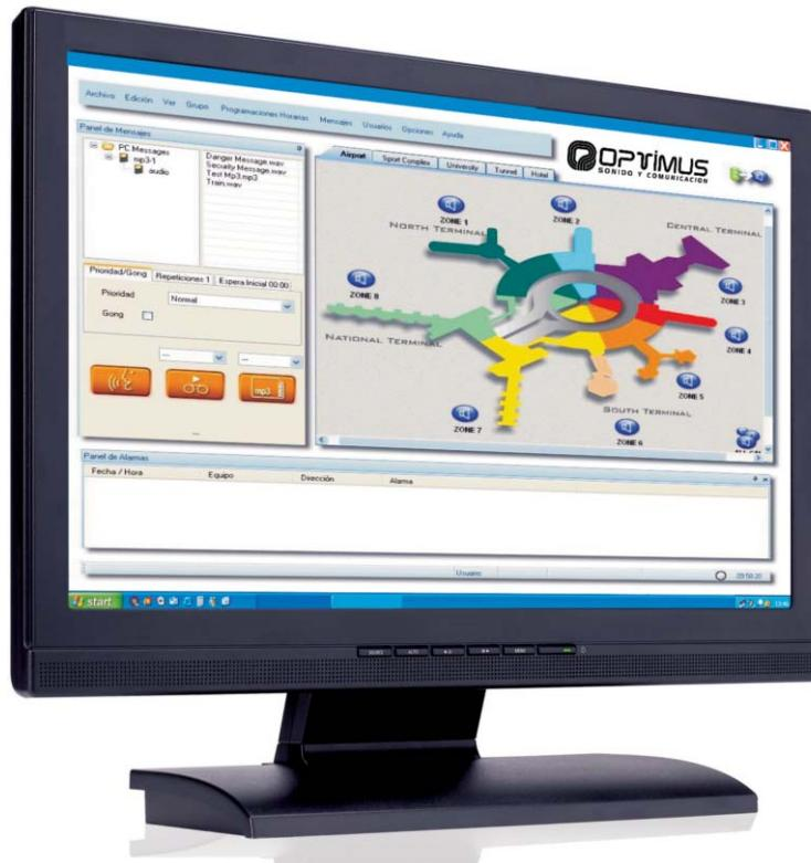
Control computers with the necessary hardware and software for managing the units of the PA control systems. The programs installed and configured in-factory for each application, allows the configuration, programming and supervision of the system.
