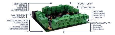
The ASD/1 contoller centralizes all access control signals (readers, locks, sensors...). The electrical supply for the devices is provided by the controller and most of the cases no additional suplly source is required.
