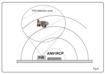
In this configuration the signal at 125 KHz, emitted by the antenna is enabled <u>only</u> when the user stands in the detection field of the sensor ( PIR or any type IR or whatever ).
