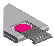
To replace the battery of the active tags, open the door by sliding it outward. Replace the coin-cell battery with an identical or equivalent: LITHIUM CR2032.
