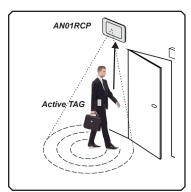
The active tag owned by the user, standing inside the field, continues the transmission each time is woken by the antenna .
