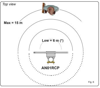
The electromagnetic field created by the antenna is roughly spherical as shown above, both on the horizontal plane and in the vertical plane. The emissions are present even behind the antenna, slighty attenuated if the fixing wall is thick
