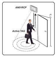
As soon as the user, carrying the active tag, enters the detection zone of 125 KHz, its tag sends a 433 MHz RF signal to the receiver which replies with a confirmation message that hushes the tag, even if it remains in the field.
