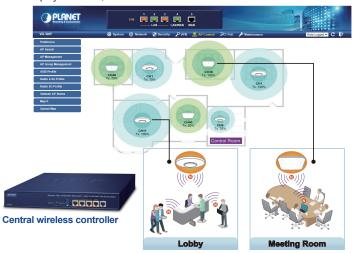
For example, to configure multiple Smart APs of the same model, the VR-300 allows clustering them to a managed group for unified management. According to requirements, wireless APs can be flexibly expanded or removed from a wireless AP group at any time. The AP cluster benefits bulk provision and bulk firmware upgrade through single entry point instead of having to configure settings in each of them separately.
